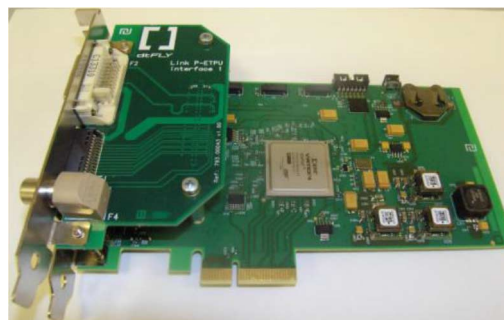
Fig. 9. Off-detector DAQ card. In the bottom of the picture the PCIe x4 connector can be easily identified. It can be seen on the left side of the picture (DAQ card front panel) how the probe IO interface is implemented as a mezzanine board allowing for the off-detector DAQ card HDMI exclusive use for future applications. The DAQ card front panel front view can be observed in Fig. 8.
