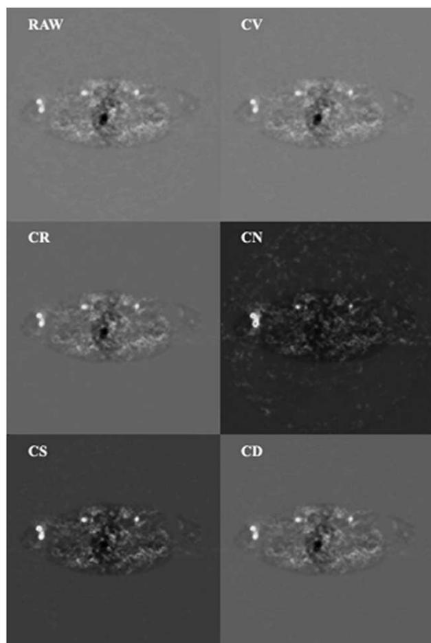
Fig. 3. Principal component image 2 based on the original values (RAW) and after application of data preprocessing: data column-wise centered (CV), data column-wise standardized (CR), data transformed as for correspondence analysis without threshold (CN), data divided column-wise by the column sum (CS) and data divided column-wise by the column standard deviation (CD).
