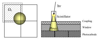
Fig. 2: The scintillation light pulse from a given crystal irradiates an area of the PS-PMT surface, which includes several photocathodes. Each of these collects and amplifies the energy, giving away a current pulse through its anode that is function of the impact location and PS-PMT properties
