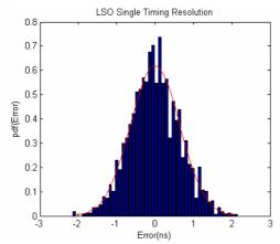
Fig. 8: LSO Single timing resolution for the implemented HW with simulated LSO pulses as input. Estimations are unbiased and limited to  $\pm 2ns$ . This enables reducing the coincidence time window to 5 ns.
