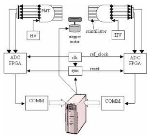
Fig. 1: Diagram of a simple tomograph with synchronized clocks for coincidence detection and a rotating gantry. A stepper motor provides the rotation of two detection heads. Each head consists of scintillator material, a PS-PMT powered by a high voltage (HV) source, acquisition electronics and the communication interface.
