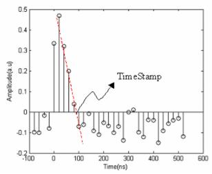
Fig. 6: Output of the implemented filter for a simulated LSO pulse. The actual zero crossing is estimated via linear interpolation.
