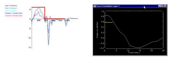
**Figure 4**. *Left:* representation of the ideal mechanical systole over the curves. *Right:* graphic representation of the cross-correlation results. The peak width is marked as the analysis accuracy indicator.
