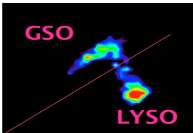
Fig. 3. Enlargement of the photopeaks area of the phoswich image of a single crystal for a field flood illumination of the array. Axis are total energy (X) and delayed energy (Y) for a selected single pixel from the matrix. Total integration time was 200 ns, delay was 140 ns
